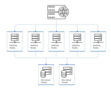
performance by offloading unnecessary SSL/ TLS from the Sitefinity back-end servers and place the burden on the LoadMaster which is optimized to handle encrypted traffic. When security is a concern, enable LoadMaster Web Application Firewall to protect Sitefinity from today's cyber threats. Finally, to deliver geographic resilience, LoadMaster's Global Server Load Balancing (GSLB) can provide automatic failover to an alternate site or cloud in the event of an outage.
